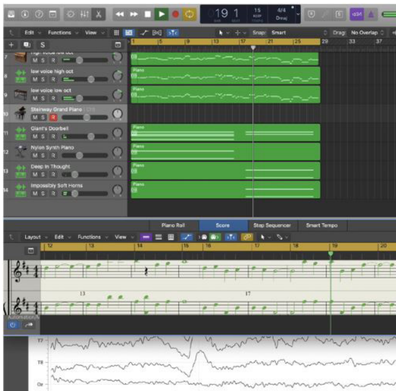
Figure 11: Top left window, MIDI score arranged for several virtual instruments within a DAW. Bottom left window, raw EEG monitor (8 channels). Right window, BCMI software using our HA-LA (blue ball) algorithm. Levels of HA-LA control the tempo of the MIDI playback, and result in different combinations of virtual instruments playing in different octaves.
