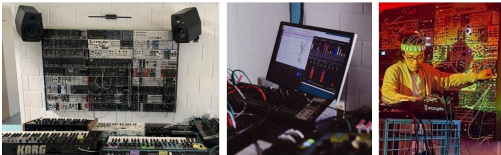
Figure 17: Left, setup of 4 analog keyboards on a table and modular system installed on a wall. Middle, EEG acquisition software and Neurosynth running side by side. Right, performer using an 8 channel EEG headband to control music, light color and head-tracking visual projection.
